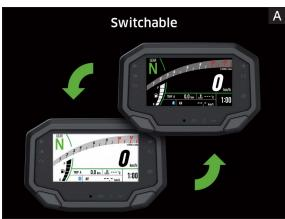
\* Display functions include: digital speedometer, digital bar-style tachometer, gear position indicator, shift lamp, fuel gauge, odometer, dual trip meters, current and average fuel consumption, remaining range, average speed, total time, coolant temperature, clock, battery voltage, Kawasaki service reminder, oil change reminder, and Economical Riding Indicator.
