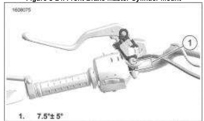
Figure 3-25. Front Master Cylinder Brake Line Location
