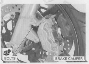
Install the brake hose eyelet to the caliper body with two new sealing washers and oil bolt.
