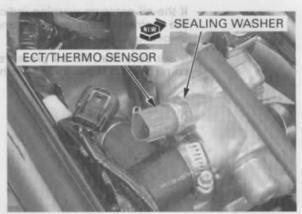
Connect the ECT/thermo sensor connector, Fill the system and bleed the air (page 7-6).
