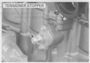
This tool can easily be made from a thin (1 mm thickness) piece of steel.
