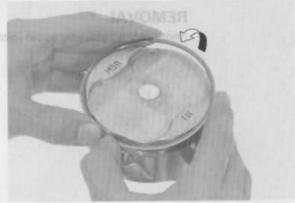
Clean carbon deposits from the ring grooves with a ring that will be discarded. Never use a wire brush, it will scratch the groove.
