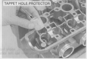
Install the valve spring seats. Install the new stem seals.
