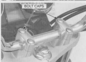
Remove the handlebar upper holder bolts, upper holders and handlebar.
