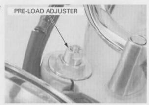
PRE-LOAD ADJUSTER ADJUSTABLE RANGE: 6 – 21 mm (0.2 – 0.8 in) from top of fork bolt PRE-LOAD ADJUSTER STANDARD POSITION: 14 mm (0.6 in) from top of fork bolt or 4th groove from top
