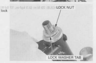
Remove the steering stem bearing adjusting nut using the special tool.
