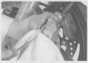
Remove the pad pins, pad spring and brake pads.
