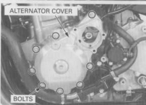
Route the alternator wire properly (page 1-23). Connect the alternator 3P (Natural) connector. Install the following:
