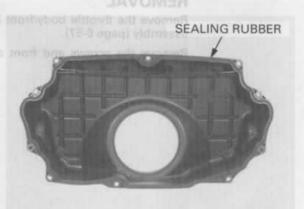
Install the front air cleaner housing to the throttle body.
