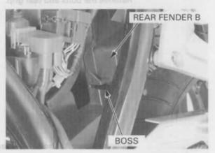
Route the main wire harness into the groove of the rear fender B, then lift up the rear fender B.
