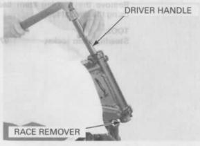
Temporarily install the steering stem nut onto the stem to prevent the threads from being damaged when removing the lower bearing inner race from the stem.
