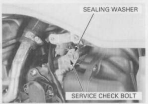
Remove the service check bolt and sealing washer, then attach the fuel pressure gauge.
