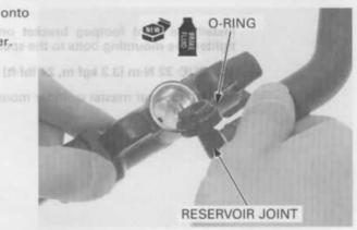
Secure the reservoir joint with snap ring.
