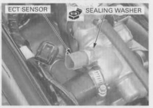
Connect the ECT sensor connector.
