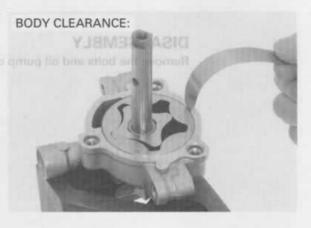
Measure the rotor tip clearance.
