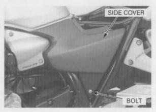
Install the side cover while aligning its tabs with the grommet on the fuel tank and frame. Install and tighten the mounting bolt securely. Install the seat (page 3-4).
