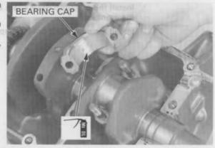
Apply oil to the bearing cap nut threads and seating surfaces and install the cap nuts.
