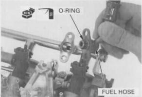
Install and tighten the fuel hose mounting bolts while holding the fuel rail.
