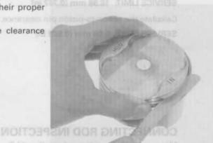
Insert the piston ring squarely into the bottom of the cylinder and measure the ring end gap.
