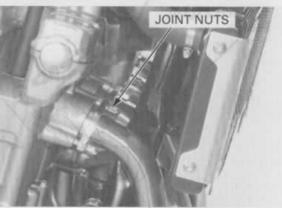
Remove the exhaust pipe mounting bolt/nut and washer, then remove the exhaust pipe.
