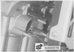
Install the washer, Install the exhaust pipe, temporarily install the | bolt and nut prop- exhaust pipe joint cap nuts, mounting washer and erly. mounting bolt/nut.
