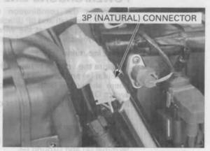
Connect the speed sensor 3P (Natural) connector.
