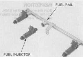
Install the fuel rail assembly onto the throttle body, being careful not to damage the seal rings.
