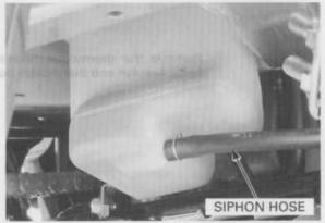
Fill the system with the recommended coolant through the filler opening up to filler neck.
