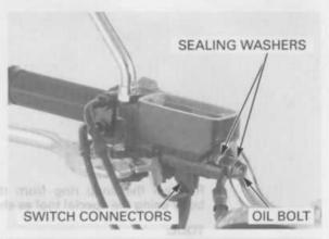
Remove the bolts from the master cylinder holder and remove the master cylinder assembly.
