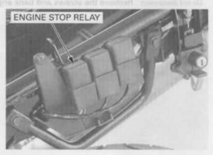
Connect the ohmmeter to the engine stop relay connector terminals.
