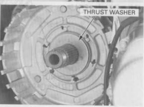
Install the clutch damper rubbers and clutch center boss into the clutch center.
