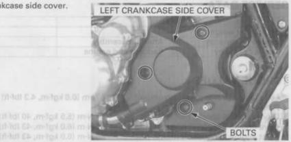
Remove the clutch slave cylinder (page 10-13). Remove the water pump assembly (page 7-15). Remove the bolts and left crankcase rear cover.
