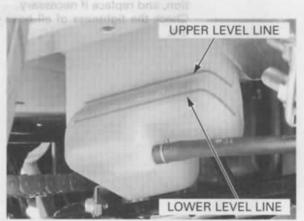
Remove the reserve tank filler cap and fill to the "UPPER" level line with 50/50 mixture of distilled water and antifreeze.
