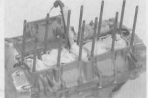
Apply molybdenum disulfide oil to the piston pin outer surface.
