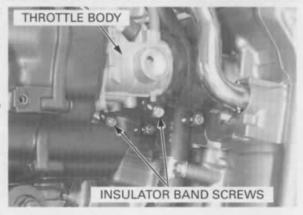
Loosen the engine side insulator band screws and remove the insulators from the cylinder head.
