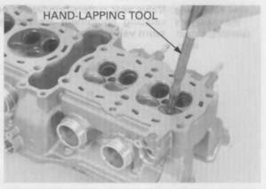
Remove the valve and inspect the valve seat face. The valve seat contact should be within the specified width and even all around the circumference.
