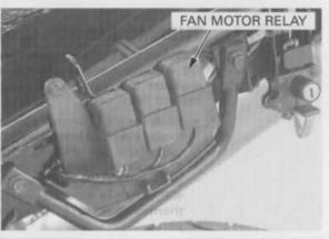
Connect the ohmmeter to the fan motor relay connector terminals.
