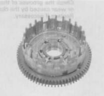
Measure the O.D. and I.D. of the clutch outer guide.
