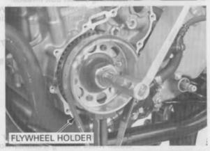
Install the starter idle gear and idle gear shaft.
