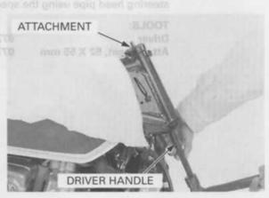
Remove the lower bearing outer race using the special tool.
