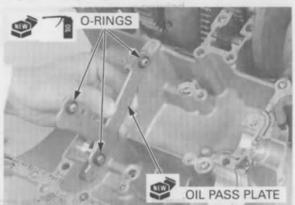
Install the oil pass pipe plate onto the upper crankcase.
