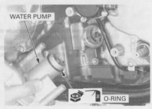
Connect the water pump-to-water joint hose to the water pump and tighten the clamp screws.
