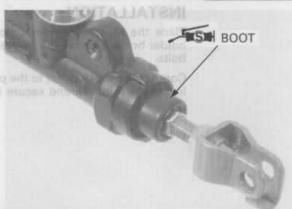
Apply brake fluid to a new O-ring and install it onto the reservoir joint. Install the reservoir joint into the master cylinder.
