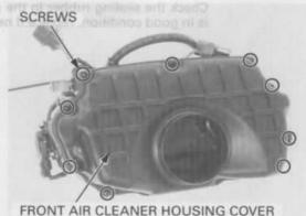
Remove the screw and MAP sensor bracket from the front air cleaner housing.
