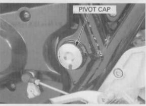
Remove the swingarm pivot nut.
