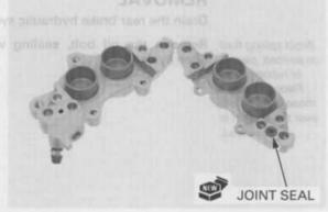
Assemble the caliper halves.
