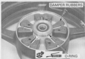
Install the driven flange assembly into the left wheel hub.
