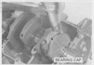
Remove the nuts and bearing cap. Measure the compressed plastigauge at its widest point on the crankpin to determine the oil clearance.
