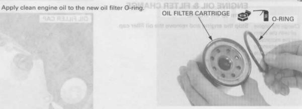
Install the new oil filter and tighten it to the specified torque.
