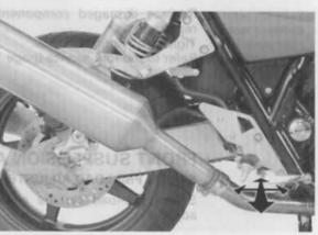
TURN CLOCKWISE: Increase the spring pre-load TURN COUNTERCLOCKWISE: Decrease the spring pre-load
