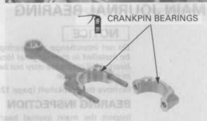
Insert the connecting rod from the cylinder side.
