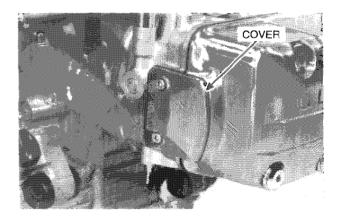
Remove the cylinder head cover.
