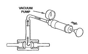
Connect a vacuum pump as shown.
