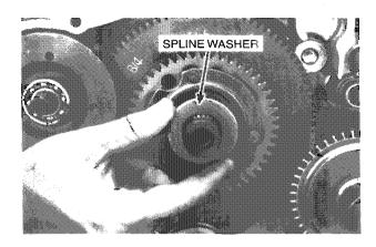
Install the oil pump sprocket, drive chain, and primary driven gear boss as an assembly.
