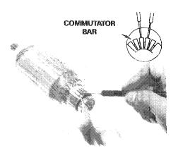
Check for continuity between the commutator bars and armature shaft. There should be no continuity.
