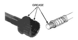
Insert the drive shaft into the pinion joint spline grooves.
