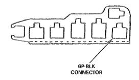
Check for continuity between each terminal as shown below and ground. There should be continuity at each gear position.
