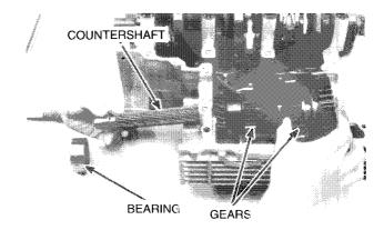
Turn the inner race of each bearing with your finger. The bearings should turn smoothly and quietly. Also check that the bearing outer race fits loosely in the crankcase.
