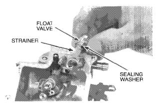
Install the float valve into the valve seat.
