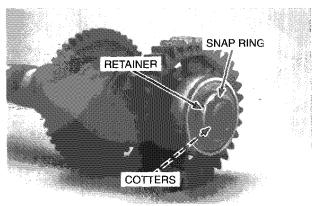
Press the output shaft out of the bearing.
