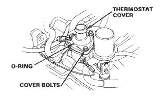
Remove the thermostat from the thermostat housing.
