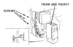
Release the antenna wires from the clamp. Remove the bolts, clamp and antenna base from the trunk.
