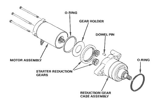
Install the dowel pin into the gear case.
