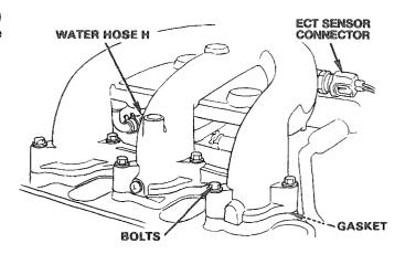
Disconnect the vacuum tube (No. 1, No. 6 GRN) and water hose H from the left intake manifold.
