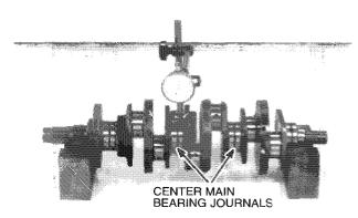
Measure the crankshaft main bearing journals and crankpins with a micrometer for out-of-round and taper.
