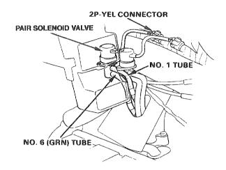
Connect a vacuum pump as shown.
