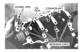
Apply oil to the main journal cap bolt threads and flange surfaces.
