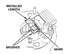
Heat the soldering iron (Capacity: about 32 W). Use low-temperature (180°-200°F) solder to solder the new brushes.
