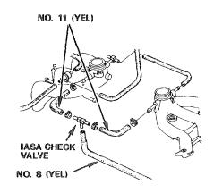
Connect a vacuum pump as shown.
