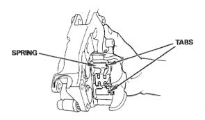
Install the new pads in the caliper.
