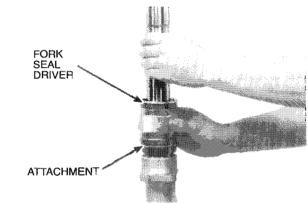
Install the stopper ring and dust seal.
