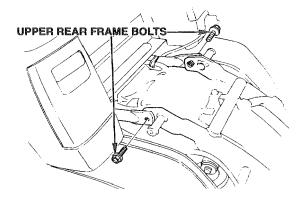
Push the rear frame forward. Tighten the lower rear frame bolts (each side).
