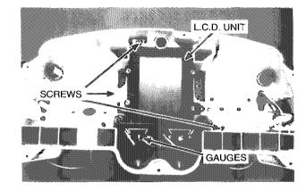
If you want to remove just the L.C.D. unit, remove ten screws. Then remove the L.C.D. unit from the base.
