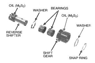
Check the shift gear for rotation.
