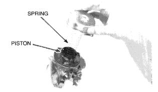
Push the jet needle holder down and turn it counterclockwise 90 degrees with an 8 mm socket. Then remove the needle holder, spring, spring holder, jet needle and washer from the vacuum piston.
