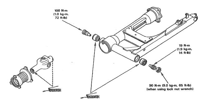
Lubricate the universal joint splines with grease.
