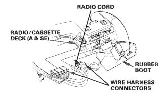
Push the lever and remove the radio/cassette deck cover from the top compartment.
