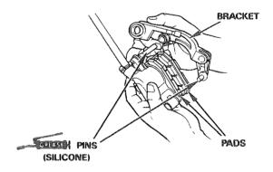
Install one pad pin. Then push the pads to compress the pad spring while you install the other pin.
