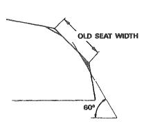
Install a 45 degree finish cutter and cut the seat to the proper width.
