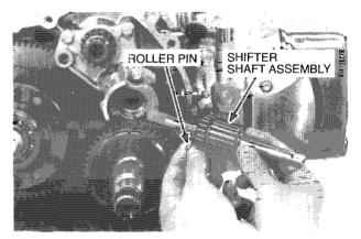
Remove the snap ring and disassemble the shaft assembly.
