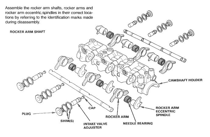
Clean the camshaft holder thoroughly. Blow through all holes and passages with compressed air.
