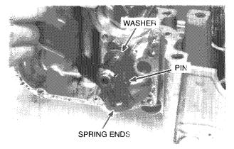
Install the shift spindle onto the left engine case and install the shift arm (smaller), aligning the arm with the spindle groove as shown.
