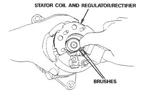
Install the rear cover on the regulator/rectifier and align the marks on the front and rear covers while moving the stator coil.
