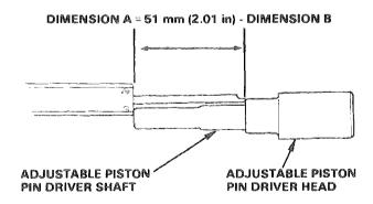
Press in the piston pin again in the same manner until the driver pilot bottoms.
