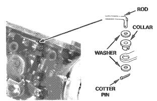
Install the washer, spring, collar, accelerator pump arm, washer, and a new cotter pin on the accelerator rod.
