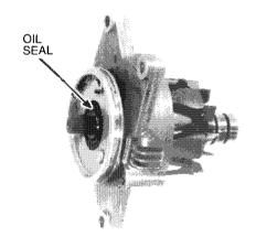
Apply grease to the oil seal lip and press a new oil seal into front cover A as shown.
