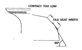
Refinish the seat to specifications, using a 45 degree finish cutter.
