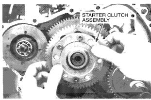
Install the bearing, washer, and starter clutch bolt.
