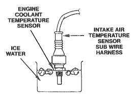
Cool the test engine coolant temperature sensor in the ice water for approximately ten minutes.
