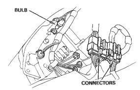
For L.C.D. unit illumination replacement only: Remove the L.C.D. unit as shown.
