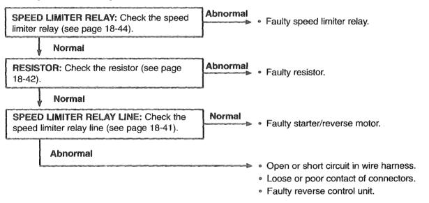
Reverse operation is rough, or reverse motor runs poorly.
