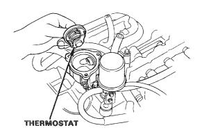
Suspend the thermostat in heated water and watch for valve opening and closing. Use an electric heating element to heat the water.
