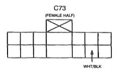
If yes, check WHT/BLK and YEL/RED circuit for an open or WHT/BLK wire between C73 & instrument panel for an open.
