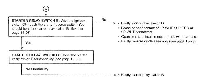
The starter/reverse motor turns in neutral position, but does not turn in gear with the side stand up and the clutch lever pulled in.
