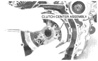
Place spring seat A, the clutch spring, and spring seat B on the clutch center and compress the spring in a press just enough to install the circlip.
