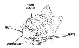
Install and tighten the three screws securely with the wire clamp.
