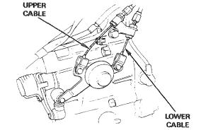
Remove the shift arm bolt and collar.
