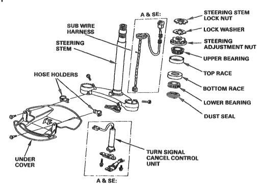
Pack the bearing cavities with grease.
