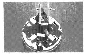
Check the continuity between the motor cable terminal and brushes with insulated wire. There should be continuity.
