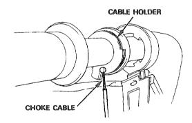
Install the left switch housing to the handlebar, aligning the boss of the housing with the hole in the handlebar.
