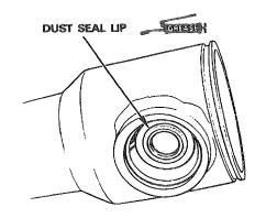
Pack the tapered roller bearings with grease. Apply grease to the bearing dust seal lips.
