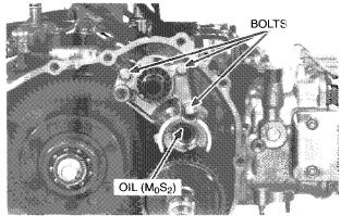
Apply oil to the needle bearings.
