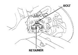
Push the piston all the way in to provide clearance for the new brake pads.
