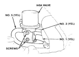
Connect a vacuum pump as shown.
