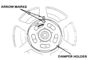
Replace the rubber dampers if they are damaged or deteriorated.
