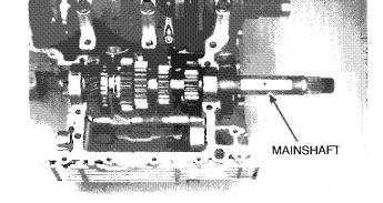
Unstake the mainshaft front bearing lock nut with a drill or grinder.
