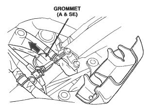
Remove the retaining screws and move the turn signal cancel control unit enough to disconnect the unit connector.
