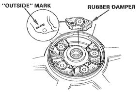
Install the damper holder into the wheel hub.
