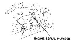
The engine serial number is stamped on the rear right side of the engine case.
