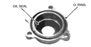
Drive the oil seal out of the holder. Drive a new seal into the holder.
