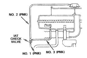
Connect a vacuum pump to the No. 2 (PNK) port of valve as shown. Plug the No. 3 (PNK) port.
