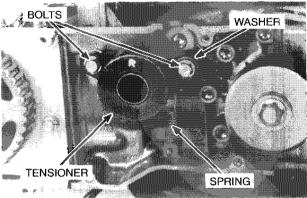
Check that the "UP" marks on the driven pulleys align with the shield cover index marks. The pulley "UP" marks should face up. Loosen the tensioner bolts and install the left timing belt.
