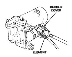
Wash the element in clean, non-flammable cleaning solvent and allow it to dry thoroughly.
