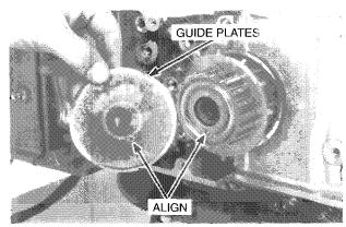
Install the washer and timing belt drive pulley bolt.
