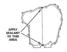
Install a new gasket and dowel pins.
