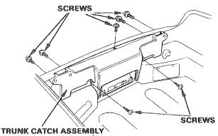
Remove the set plate and the lock cylinder. Remove the three screws and the trunk/saddlebag opener unit from the trunk.
