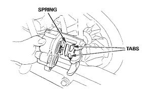
Install the new pads in the caliper.
