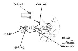
Install the spring, hooking it onto the tab of the output shaft bearing holder as shown.
