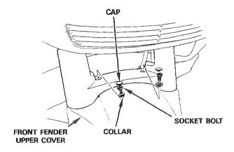
Remove two socket bolts, two flange bolts, and the collars.
