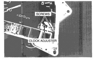
Remove two electric tachometer terminal screws and two tachometer mounting screws.
