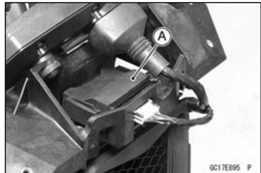
Oxygen Sensor [A] (Equipped Models)
