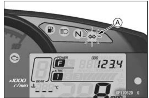
**Check 3-5: Red Warning Indicator Light (LED) (Oil Pressure Warning) Inspection**
