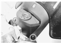
• Remove the fuel tank bracket 1.
