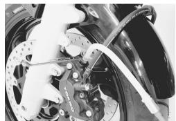
· Close the caliper air bleeder valve and disconnect a clear hose. Fill the reservoir with new fluid to the upper mark of the reservoir.
