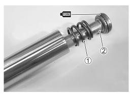
Apply THREAD LOCK "1342" to the cylinder bolt and tighten it to the specified torque using the special tools.
