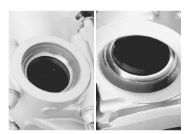
• Remove the steering stem lower bearing inner race with a chisel.
