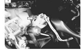
4) Disconnect the injector coupler and measure the resistance between terminals.
