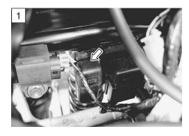
Is the cooling fan relay OK?
