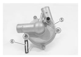
Remove the impeller securing bolt by holding the impeller with a water pump pliers.
