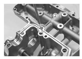
• Remove the oil jet ③ (for cam chain tension adjuster) from the cylinder head.
