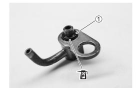
• Install each piston cooling oil jet with the bolt.
