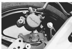
• Inspect the pad mounting pin for wear or damage. If necessary, replace it with a new one.
