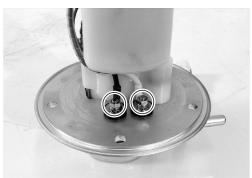
• Remove the lead wire ①, screws and fuel level gauge ②.
