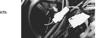
4) Disconnect the CKP sensor coupler and measure the resistance.
