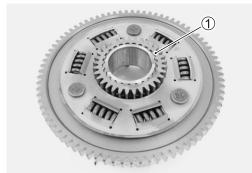
• Install the primary driven gear assembly.
