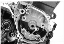
Apply SUZUKI BOND lightly to the groove of CKP sensor lead wire gromet.
