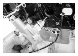
Water pump mounting bolt: 10 N⋅m (1.0 kgf-m)
