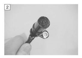
3 Check the speed sensor output voltage.
