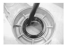
• Remove the final drive gear bearing with the special tools.
