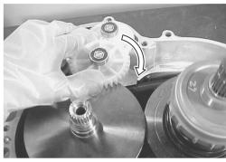
• Remove the primary slide pulley idle gear ② and ③.
