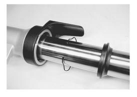
• Pull the inner tube out of the outer tube.
