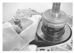
• Remove the secondary pulley assembly.
