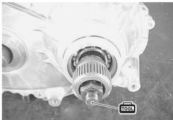
• Press in the secondary pulley shaft adaptor with the special tool.
