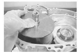
• Remove the shim 1 and O-ring 2.
