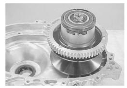
• Install the primary pulley shaft adaptor with the special tool.
