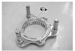
• Install the rear hub driven gear joint.
