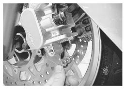
• Tighten the pad mounting pin  ${\mathfrak T}$  to the specified torque.
