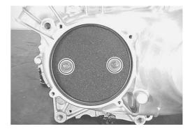
• Remove the secondary pulley shaft nut by holding the shaft with the special tools.
