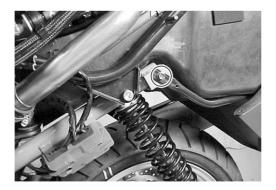
• Remove the trunk light seat switch ②.
