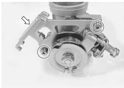
• Remove the synchronizing screws.
