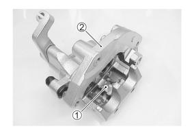
• Remove the parking brake housing 3.
