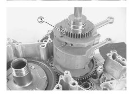
• Install the crankcase oil separator.
