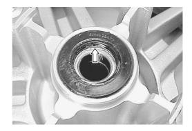
• Remove the dust seal with the special tool.
