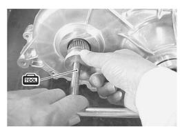
• Apply THREAD LOCK SUPER "1360" to the primary pulley shaft bolt.
