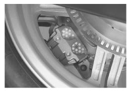
• Remove the brake lock cable guide ②.
