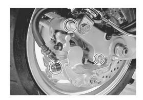
• Remove the pad spring ① and caliper holder ②.
