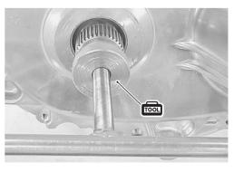
• Tighten the primary pulley shaft bolt to the specified torque with the special tools.
