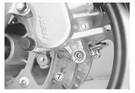
• Install the plug ® and tighten it to the specified torque.
