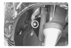
• Check the AAT sensor coupler for loose or poor contacts. If OK, measure the AAT sensor resistance.
