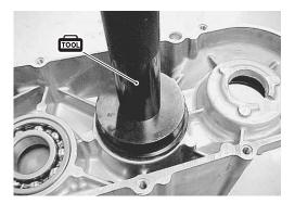
• Install the plate ② into the final gear case cover at the No.2 gear, and then install the bearing.
