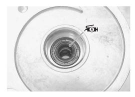
• Install the new mechanical seal using a suitable size socket wrench.
