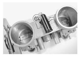
• Remove the throttle cable bracket.
