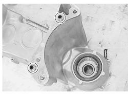
• Remove the final gear case bolts in a crisscross pattern.
