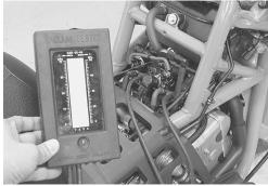
· Equalize the vacuum of the cylinders by turning each air screw 3 and keep it running at idling speed.
