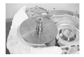
• Install the CVT belt so that the direction mark on the CVT belt points in the normal turning direction.
