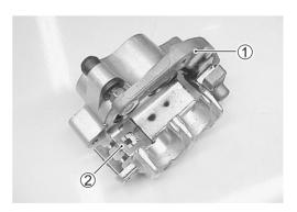
• Place a rag over the pistons to prevent them from popping out and then force out the pistons using compressed air.
