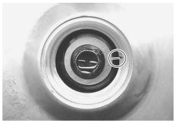
• Push the cam chain tension adjuster rod and insert the special tool.
