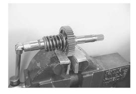
Remove the washer ®, spring stopper 9, dumper cam spring
