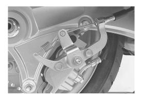
Remove the caliper 8.
