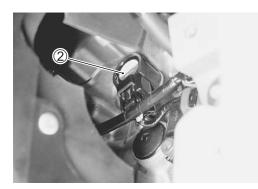
• Remove the spark plugs with the spark plug wrench.
