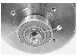
• Remove the bearing with a bearing puller.
