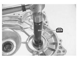
• Install the bearing retainer ①.
