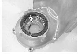
• Remove the oil seal with the special tool.
