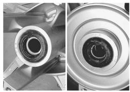
• Remove the dust seals by using the special tool.
