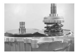
• Install the primary slide pulley idle gear 1 and 2.
