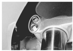
• Remove the front fork cap bolt ③ with the special tool.
