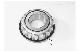
• Remove the swingarm pivot bearing with the special tools.
