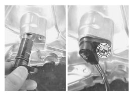
• Install the pulley position sensor ① with the sensor pushed toward the primary pulley shaft side.
