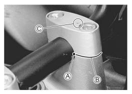
• Tighten the handlebar clamp bolt to the specified torque.
