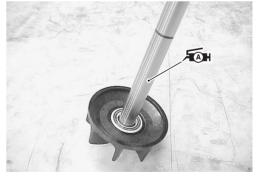
• Install the E-ring 1 to the impeller shaft.
