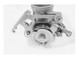
Apply a small quantity of grease to the shaft end and seal lip.
