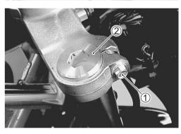
• Loosen the front fork lower clamp bolts.
