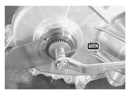
• Separate the CVT assembly by using 6 mm screws.
