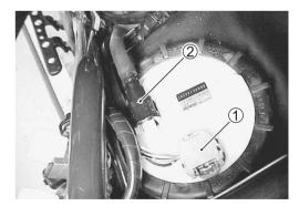
• Remove the fuel pump ring locknut by using the special tool.
