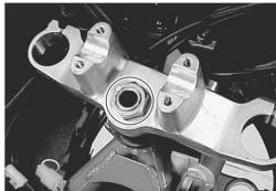
• Remove the steering stem nut with the special tool.
