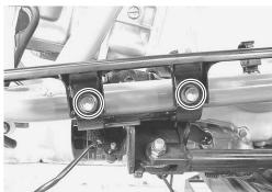
• Remove the engine from the frame.
