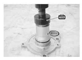
• Install the new oil seal using the special tool.
