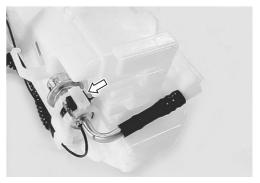
• Disconnect the fuel pump lead wire coupler and ground wire.
