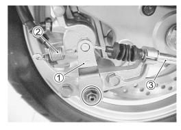
• Remove the caliper.
