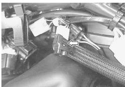
Measure the voltage between the terminals using the multi circuit tester.
