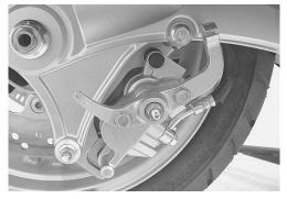
• Tighten the pad mounting pins to the specified torque.
