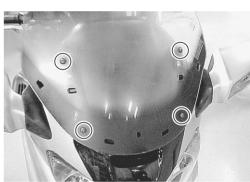
• Remove the wind screen brace 2.
