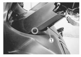
• Remove the handlebar front cover ②.
