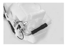
• Install the fuel level gauge.
