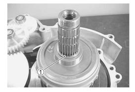
• Turn the primary slide pulley idle gear clockwise and open the primary pulley fully.
