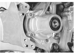
Inspect the dust seal on the bearing for wear and damage. If any defects are found, replace the bearing with a new one.
