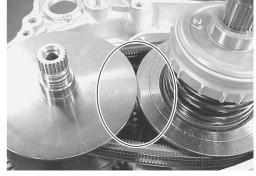
• Check that the CVT belt is in parallel with the CVT cover mating face.
