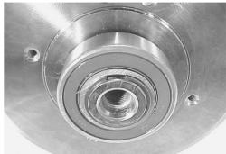
• Apply THREAD LOCK "1342" to the secondary pulley fan bolts and tighten them.
