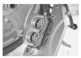
Assemble the new pads, insulators ① and shims ①.
