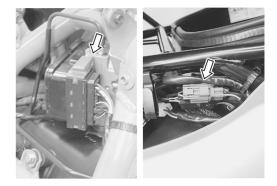
1) Check the resistance between terminal ② (B/Y) on the ABS control unit coupler and ground.
