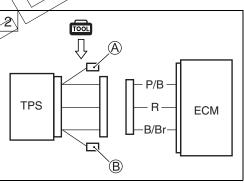
7) If OK, then measure the TP sensor resistance at the test harness terminals (between terminal © and terminal ©).
