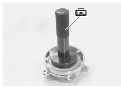
• Remove the driveshaft left bearing dust seal from the retainer using the special tool.
