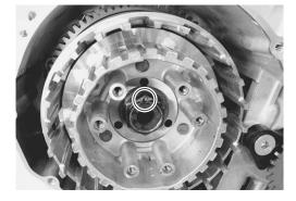
• Hold the clutch sleeve hub with the special tool.
