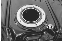
• When installing the fuel pump assembly, first tighten all the fuel pump mounting bolts lightly and then to the specified torque, in the ascending order of numbers.
