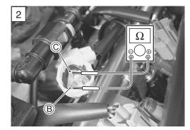
7) If OK, then measure the STP sensor resistance at the wire terminals (between BI wire C and B wire B).
