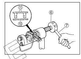
• Continue pressing the joint plate until the distance between the two joint plates come to the specification.
