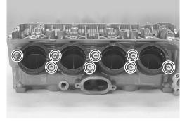
• Apply SUZUKI SUPER GREASE "A" to the O-rings.
