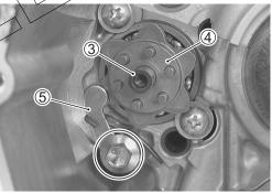
• Remove the shaft (4), bearing (5) and thrust washer (6).
