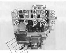
• Remove the dowel pins, O-ring 2 and cap 3.
