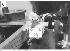
4) Then, swap the wires supplied 12 V and check the operation of EXCVA.
