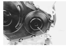
• Turn the crankshaft to bring the line (A) on the CKP sensor rotor to the rib (B) behind the clutch cover and also to bring the cams to the position as shown.
