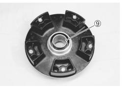
• Remove the dust seal with the special tool.
