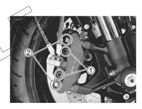
Install the spring to the caliper, bring its wider side of pawl facing top.
