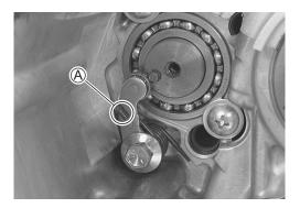
Install the starter idle gear No. 1 shaft 5, thrust washer 6, bearing 7, starter idle gear No. 1 8, washer 9, and spring washer 10.
