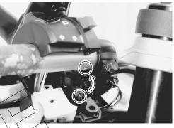
After installing the steering, the following adjustments are required before driving.
