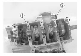
• Apply SUZUKI BOND to the mating surface of the lower crankcase.
