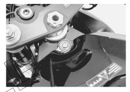
• Lift and support the fuel tank with the fuel tank prop stay
