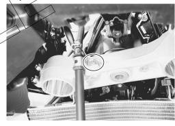
• Remove the steering stem lock-nut, washer and steering stem nut with the special tools.
