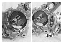
• Apply THREAD LOCK to the bolts and tighten them to the specified torque.
