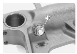
• Remove the damper rod bolt with the special tool and a hexagon wrench.
