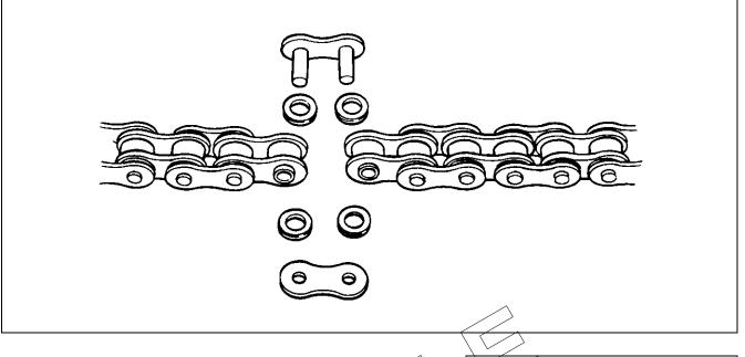
Use the special tool in the following procedures, to cut and rejoin the drive chain.
