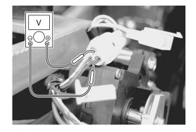
If the measured voltage is more than specification, adjust the No.2 cable adjuster as follows:
