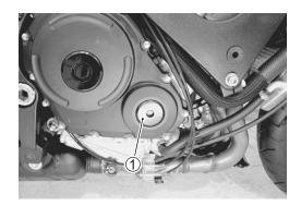
• Turn the crankshaft to bring the line (A) on the CKP sensor rotor to the rib (B) behind the clutch cover and also to bring the notches (A) on the left ends of both camshafts (Ex. and In.) to the positions as shown.
