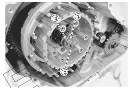
Insert the clutch drive plates and driven plates one by one into the clutch sleeve hub in the prescribed order.
