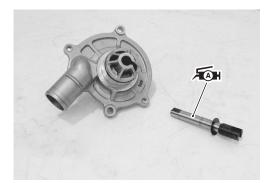
• Apply SUZUKI SUPER GREASE "A" to the impeller shaft.
