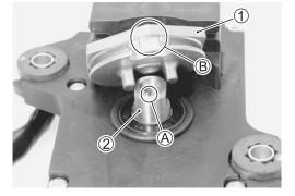
• Hold the EXCVA pulley with an adjustable wrench, and then tighten the EXCVA pulley mounting bolt to the specified torque.
