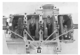
• Apply a MOLYBDENUM OIL SOLUTION to each crankshaft journal and bearing lightly.
