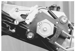
• To set the EXCV to fully close position, apply 12 V to (A) and (B) terminals.
