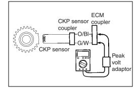
If the peak voltage is lower than the standard range, check the peak voltage at the CKP sensor lead wire coupler.
