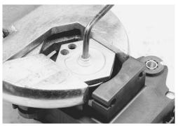
• Tighten the EXCVA mounting bolts to the specified torque.
