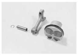
• Remove the piston pin circlip ①.
