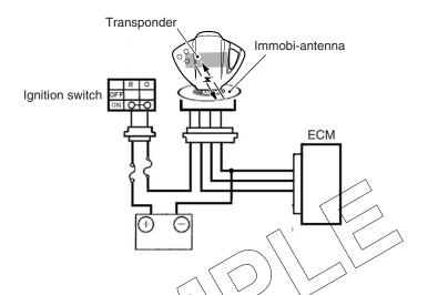
Also, when the ignition switch is turned ON, the indicator light flashes as many as the number of IDs registered in ECM. Thereafter, if the IDs are in agreement, the indicator light turns on for two seconds to notify of completion in successful communication.
