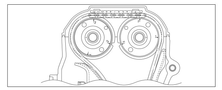
• Install the dowel pins.
