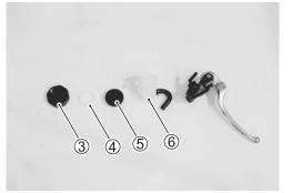
• Remove the brake switch (7) and brake lever (8).
