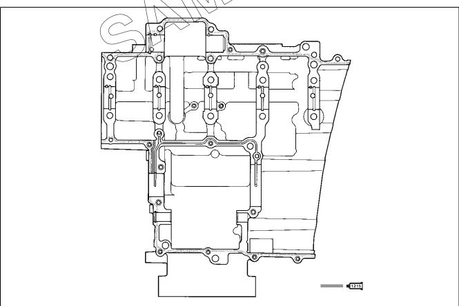
• Tighten the crankshaft journal bolts (M9) in ascending order of numbers assigned to these bolts. Tighten each bolt a little at a time to equalize the pressure in the following two steps.
