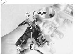
• Install the fuel injector (5) by pushing it straight to the delivery pipe (6).
