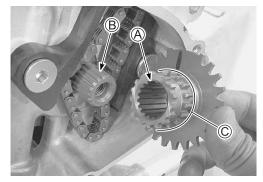
• While holding the generator rotor with the special tool, tighten the CKP sensor rotor/cam chain drive sprocket bolt.
