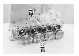
• Install the pistons and conrods into the cylinders from upside.
