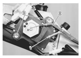
• Hold the EXCVA pulley with an adjustable wrench, and loosen the pulley mounting bolt.
