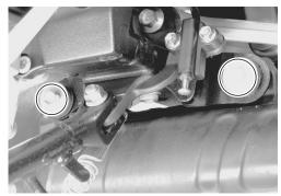
• Tighten the radiator mounting bolts to the specified torque.
