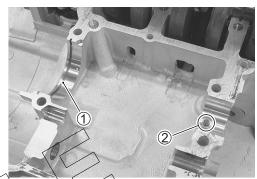
• Install the countershaft assembly to the upper crankcase.
