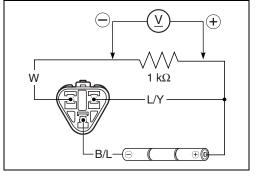
6) Under this condition, if a suitable screwdriver touching the pick-up surface of the CMP sensor is moved, the tester reading voltage changes (0.8 V and less ↔ 4.3 V and more).
