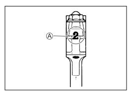
• Check the corresponding crank pin O.D. code number ("1", "2" or "3") <sup>(B)</sup>.
