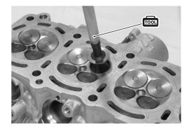
• If the seat width (1) measured exceeds the standard value or seat width is not uniform, reface the seat using the seat cutter.
