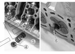
• Remove the oil seal  ${\mathcal T}$  and spring seat  ${\mathfrak B}$
