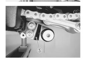
• Remove the brake fluid reservoir mounting bolt.
