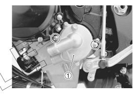
• Remove the water pump cover 2 and ai bleeder plug 3.
