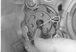
• Install the washer 6 and gearshift shaft assembly 7.
