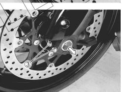
• Raise the front wheel off the ground and support the motorcycle with a jack or a wooden block.
