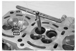
Cool down the new valve guides in a freezer for about one hour and heat the cylinder head to 100 °C – 150 °C (212 °F – 302 °F) with a hot plate.
