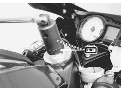
• Remove the dust seal cover ①, dust seal ②, steering stem upper bearing inner race ③ and bearing ④.
