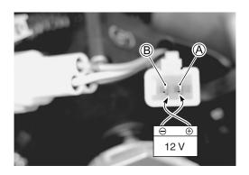
Measure the position sensor output voltage at fully open position.
