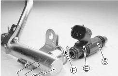
• Install the fuel delivery pipe assembly ⑦ to the throttle body assembly.
