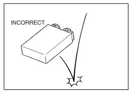
• Be careful not to touch the electrical terminals of the ECM. The static electricity from your body may damage this part.
