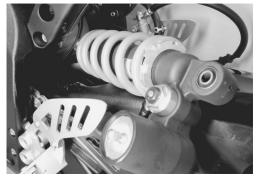
• Remove the rear shock absorber.
