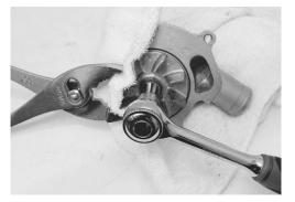
• Remove the mechanical seal ring ④ and rubber seal ⑤ from the impeller.
