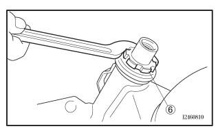
b. Loosen the lower ring nut ④ and then tighten it to specification with a ring nut wrench ⑤.
