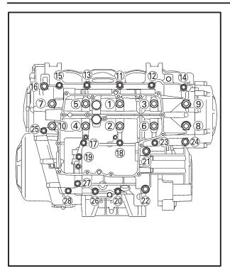
f. Tighten the bolts to specification in the tightening sequence cast on the crankcase.
