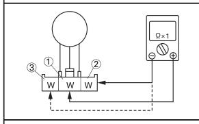
• Measure the stator coil resistances.
