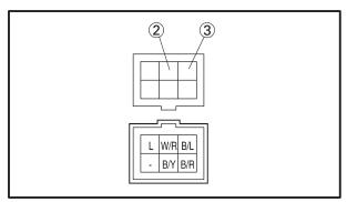
Connect the battery to the EXUP servomotor connector and check if the servomotor operates properly.
