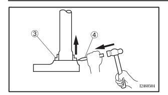
b. Remove the bearing race ③ from the lower bracket with a floor chisel ④ and hammer.
