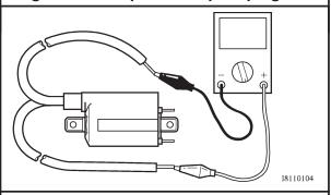
• Measure the secondary coil resistance.
