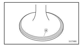
a. Apply a coarse lapping compound ⓐ to the valve face.
