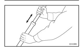
9. Slowly stroke the inner tube ② up and down to distribute the fork oil once more (1 stroke = about 150 mm).
