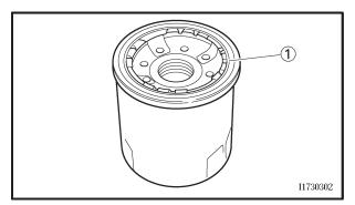
b. Apply a thin coat of engine oil onto the O-ring1) of the new oil filter cartridge.
