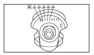
For example, if the crankcase " $J_1$ " and crankshaft web " $J_1$ " numbers are "6" and "2" respectively, then the bearing size for " $J_1$ " is:
