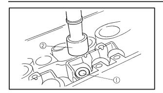
e. Install the new valve pad 1 and the valve lifter 2.
