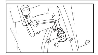
c. Turn the throttle stop screw ② in direction ③ or ⓑ until the specified engine idling speed is obtained.
