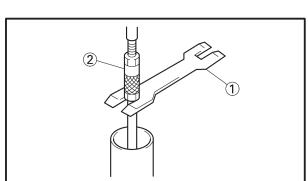
a. Install the fork spring, spring seats, and spacer.
