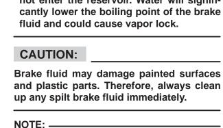
In order to ensure a correct reading of the brake fluid level, make sure that the top of the reservoir is horizontal.
