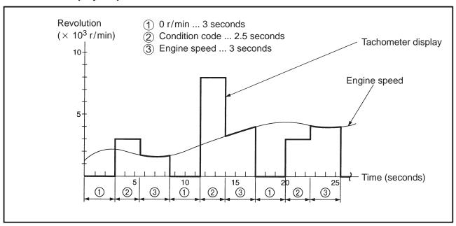
When more than one item is being monitored, the tachometer needle displays the condition codes in ascending order, cycling through the sequence repeatedly.
