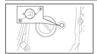
b. Check that the mark ⓐ is within the required firing range ⓑ on the pickup coil rotor.
