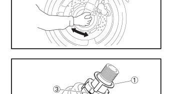
a. Remove the lock washer ①, the upper ring nut ②, and the rubber washer ③.
