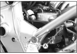
• Loosen the nuts [A] and remove the ABS hydraulic unit [B] from the bracket [C].
