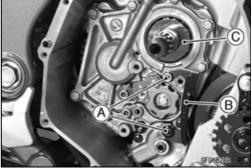
• Remove the oil pump sprocket bolt [A].
