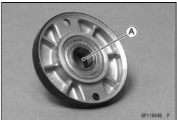
• Apply thin coat of grease to the oil seal [A].
