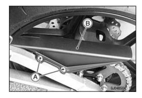
• Using a suitable tool, replace the drive chain. Recommended Tool - DID Chain Joint "ZJ"
