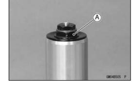
• Install the fork spring compressor as shown in the figure.
